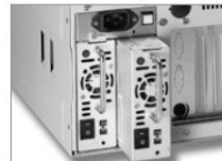
Optional hot-swap redundant power supply
